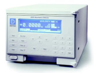
The Dionex AD25 is a dual beam, variable wavelength absorbance detector for Dionex Ion and Liquid Chromatography Systems. Broad spectral capability is provided by two light sources: a deuterium lamp for ultraviolet wavelengths, and a tungsten lamp for visible detection. Validation of wavelength accuracy is accomplished efficiently using a built-in holmium oxide filter test. The AD25 can be operated at the front panel or automated with Dionex chromatography software.
